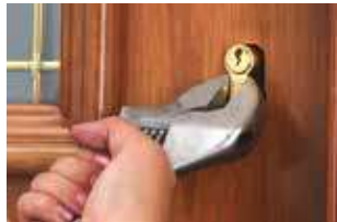
B. Tighten up with a switch wrench and swing it. (cylinder is exposed by at least 10mm).
